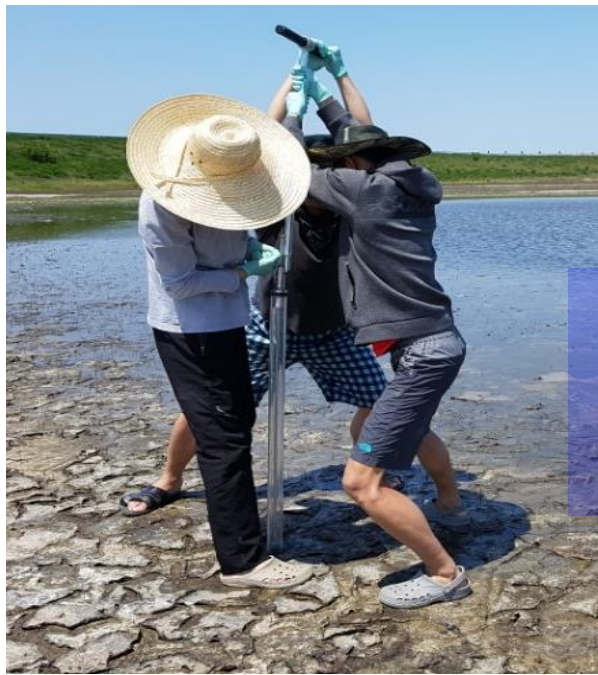
Current sediment coring (max depth: ~1 m)
